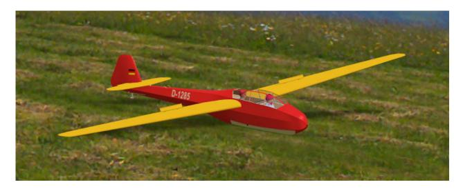
The smallest REFLEX model weighs 6 lb what is easily achievable in reality at that size (130 in). The setup is "the other way around". The static stability margin was reduced to 10%, giving a 1.02 pitch damping ratio. In the simulator, the model behaves noticeably different from the bigger version.
