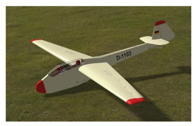
Accordingly, the two smaller REFLEX models have a SD 7062 airfoil, which is rather thick (14% what allows for a lightweight wing) but has super-critical airflow already at smaller Re numbers. The Goe 769 airfoil for the bigger REFLEX model is rather similar to the original's Mü 14.5, not only in thickness but also in shape and characteristics. Maybe the model would need trip strips, but it should behave similar to the original (also regarding the pitching moment) and perform decently.
