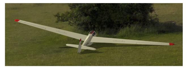
Given the true-to-scale small stabilizer, low weight and small static stability margin (moment of inertia) are necessary to achieve a greater than 1 pitch damping ratio. Accordingly, the "light" 1:3.5 scale version flies best. The assumed 11 lb weight (to stay below the 5 kg weight limit for flying off airfields
