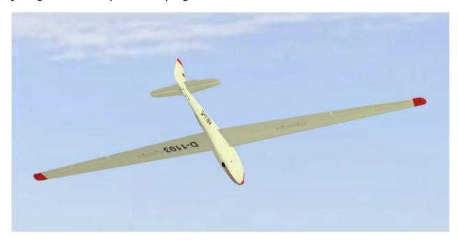
The 15% static stability margin was not changed for the "medium" (15.75 lb) and the "heavy" (19.75 lb) versions. Due to the bigger moments-of-inertia, the pitch damping ratio is reduced to 0.88 and 0.78, respectively. That would be still not bad for an aerobat, but what that means for a soarer can be tried out in REFLEX.
