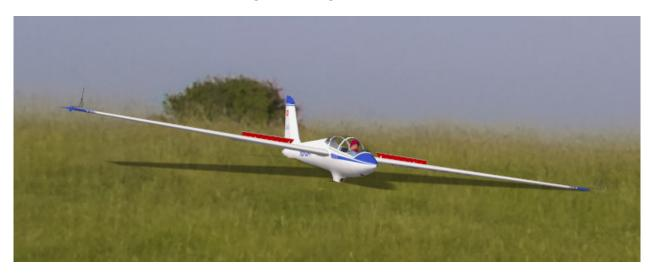
The wings are really thin, 12% on the original and as shown here, only 8.7% on the model with the MH-32 airfoil. Spoilers are only at the wing top.
