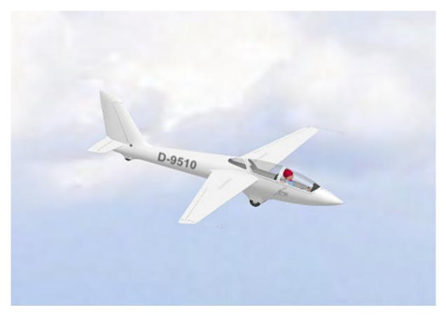
Well visible in the side view are the mid-wing configuration as well as the tail-wheel landing gear. The main wheel's axle sits exactly below the wing's leading edge. That's in accordance with an old rule-of-thumb used full-size as well as in modeling.
