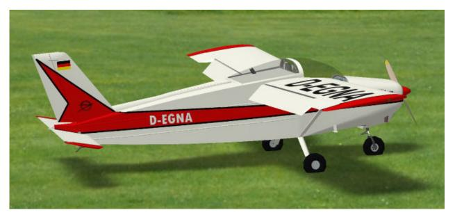
For comparison, there's an "expert" setup of the big version with the ZG 45 (because it's closest to the real thing), with 35 degrees flap deflection and 15 degrees elevator. This setup spins without any trick and may be fully flared for landing. But you may notice that you really have to be an expert (or practice) to do this properly. The picture shows full flaps and full up elevator as well as the paint scheme used for the first airplanes built in the 1960s.
