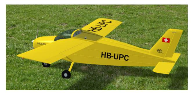
The model's propeller is a wooden Master Airscrew, mainly because I had it, but also because a wooden propeller is well suited to the gas engines used. The original aircraft has grey or black colored metal propellers. The spinner is aluminum colored just because I like that more than a yellow one.
