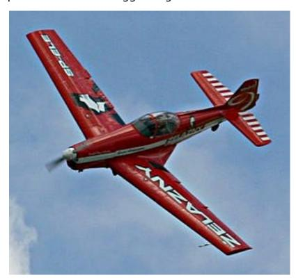
The wing was clipped to enhance the roll rate. To this end it was as well necessary to supplement the now smaller ailerons with additional inner ailerons (see picture). The split flaps used on the trainer had to be cancelled, but it's easy to do without any flaps.
