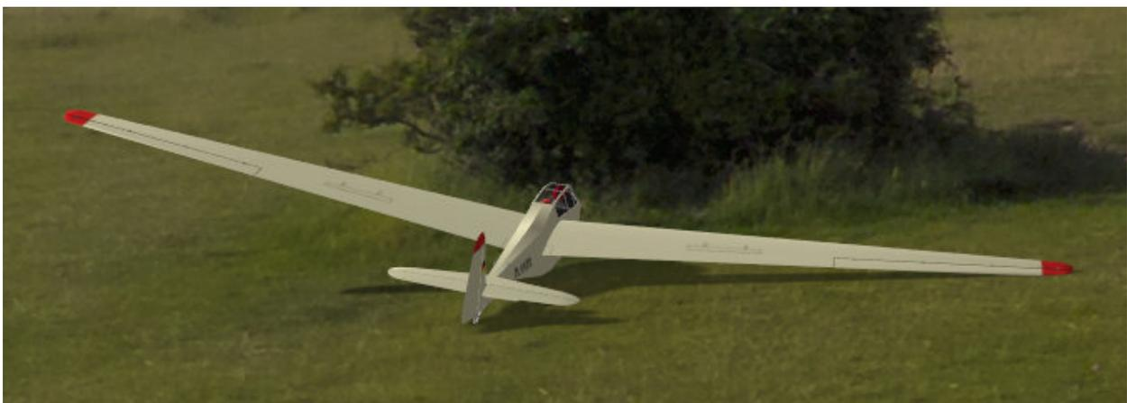
Given the true-to-scale small stabilizer, low weight and small static stability margin (moment of inertia) are necessary to achieve a greater than 1 pitch damping ratio. Accordingly, the "light" 1:3.5 scale version flies best. The assumed 11 lb weight (to stay below the 5 kg weight limit for flying off airfields
