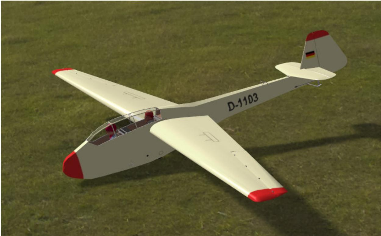
Accordingly, the two smaller REFLEX models have a SD 7062 airfoil, which is rather thick (14% what allows for a lightweight wing) but has super-critical airflow already at smaller Re numbers. The Goe 769 airfoil for the bigger REFLEX model is rather similar to the original's Mü 14.5, not only in thickness but also in shape and characteristics. Maybe the model would need trip strips, but it should behave similar to the original (also regarding the pitching moment) and perform decently.
