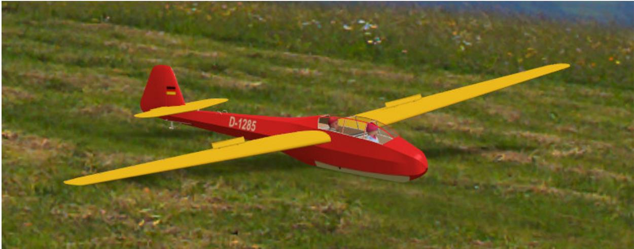
The smallest REFLEX model weighs 6 lb what is easily achievable in reality at that size (130 in). The setup is "the other way around". The static stability margin was reduced to 10%, giving a 1.02 pitch damping ratio. In the simulator, the model behaves noticeably different from the bigger version.
