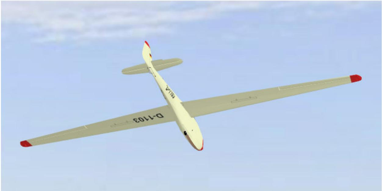
The 15% static stability margin was not changed for the "medium" (15.75 lb) and the "heavy" (19.75 lb) versions. Due to the bigger moments-of-inertia, the pitch damping ratio is reduced to 0.88 and 0.78, respectively. That would be still not bad for an aerobat, but what that means for a soarer can be tried out in REFLEX.
